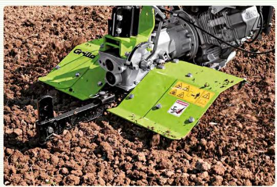
The user can adjust **the tilling depth** by putting more or less pressure on the spur and adjusting its height. If the spur is adjusted to a higher position, the balance of the machine is shifted onwards so it will go forward easily and it will consequently not work very much into depth. On the contrary, if the spur is adjusted to a lower position, the machine will tend to work on the spot, allowing therefore a deeper tilling of the soil.
