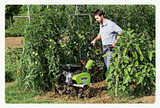
**The side discs** are necessary to balance the machine and to mark out the tilled area. When working on softer soil, the side discs are recommended to prevent the tilled soil from covering the new plants and damaging their roots.
