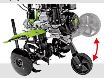
The side wheels are an optional accessory. Extremely practical for long transfers, they are quickly assembled and driving is provided by the motion of the tiller (all Princess models, 3500 and 11500).
