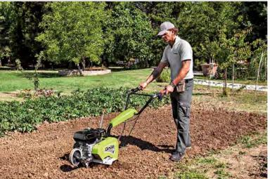
The furrower allows to make regular **furrows** with adjustable width and depth.
