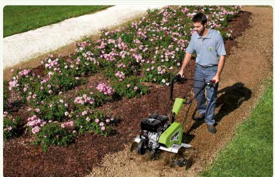
On **soft soil** the side discs ensure good flotation and allow the machine to move forward easily without sinking. **If the soil is hard** or wet, it is recommended to use the tiller without side discs to allow the tines to reach deeper into the ground.
