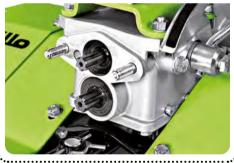
The **spur** is swinging and heightadjustable in 8 positions. The adjustable furrower is attached once the spur has been removed and allow to carry out furrows of different widths.
