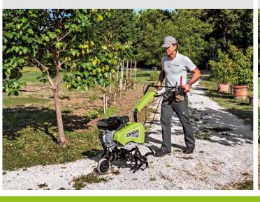
To obtain **a perfect finishing** and avoid walking on the tilled soil, all Grillo rotavators have a sideway adjustable handlebar.
