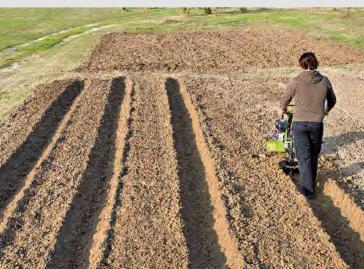
On very **hard soil** it is recommended to turn the spur to the front and to work without side discs.
